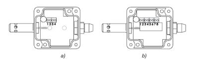
Fig. 5. Marking of the terminals for the connection of external signals of the P18(D) transducers in versions: a) without analog outputs, b) with analog outputs.
