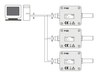
Fig. 13. Connecting the RS-485 interface.
