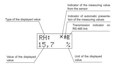
Fig. 7. Description of the P18D transducer readout field
