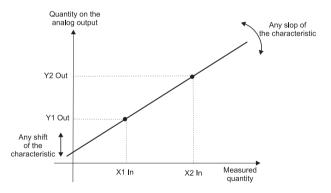
Fig. 11. Individual characteristic of analog output
