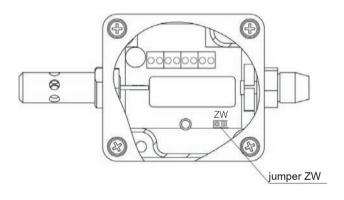
Fig. 13. Placement of the jumper setting temporary communication parameters
