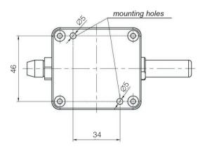
Fig. 4. Lay-out of mounting holes of the P18(D) transducer
